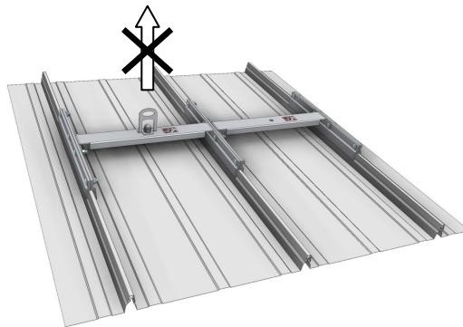
The **LUX-top® GBD** anchor device is approved for simultaneous use by **3 people** with full body harnesses and energy absorbers (including 1 person for first aid/rescue).
