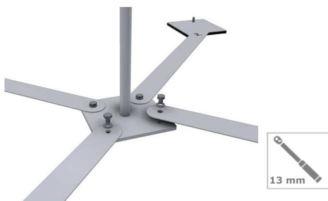
Fig. 3: Bolting the feet
