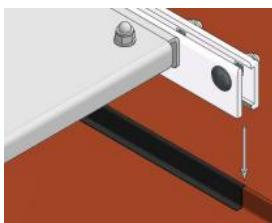
Mounting on copper only permitted with EPDM-stripes (as a separating layer) available at ST Quadrat!
